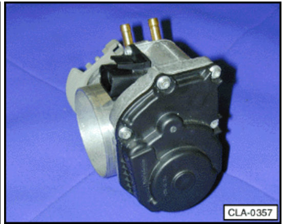
J338 Throttle valve control module (2.8 ltr. engine)
