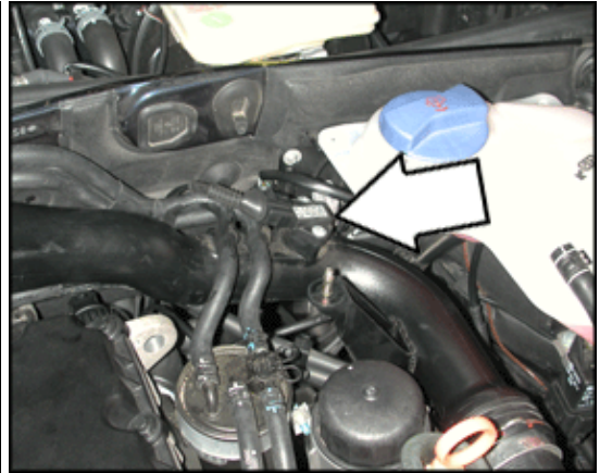
G42 Intake Air Temperature (IAT) Sensor (2.0 ltr. tdi engine)
