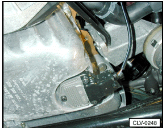
G266 Oil level thermal sensor (1.8 ltr. engine)
