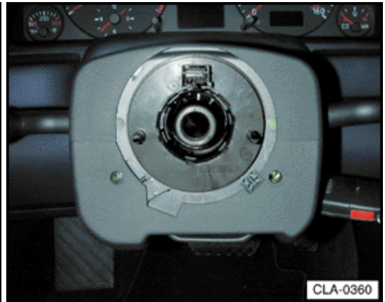
F138 Airbag spiral spring/return spring with slip ring
